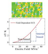
By internal biasing a relaxor ferroelectric polymer, it is demonstrated numerically and experimentally that both electrocaloric effect and electrocaloric coefficient can be enhanced. This approach provides a general route to enhance low-field electrical performances of such square-rule materials and thus pave the way to develop smart electroactive devices with better electrical reliability and safety.
