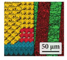
Perovskite thin films are deposited on Si substrates covered with inorganic nanosheets of  $Ca_2Nb_3O_{10}$  or  $Ti_{0.87}O_2$ . These nanosheets are used to control the nucleation of films that consist of a SrTiO2 buffer layer and a SrRuO<sub>3</sub> top layer. The two types of nanosheets are micropatterned to locally tailor the crystallographic orientation, allowing lateral control of the magnetic properties of SrRuO<sub>3</sub>.
